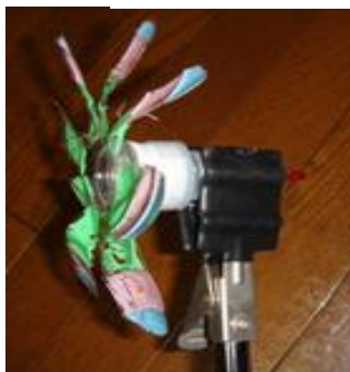
風力発電 LED 点灯
